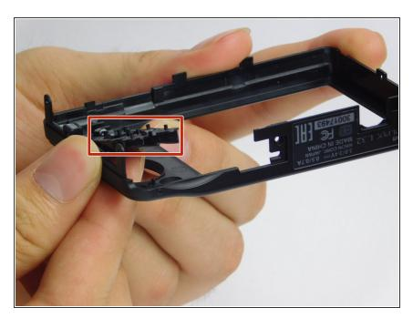
Secure the black back case in hand and remove selection buttons from the case by pushing them upward and replace them with a new set of buttons.
