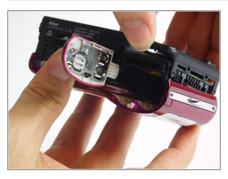
Open the battery compartment door and pull the black back face apart from the front red face.
