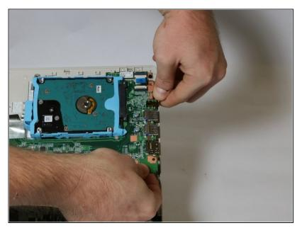
Lift on the motherboard from the USB port area while pulling the frame away from motherboard.
