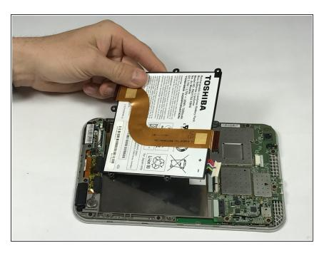
Battery will lift out of the device.
