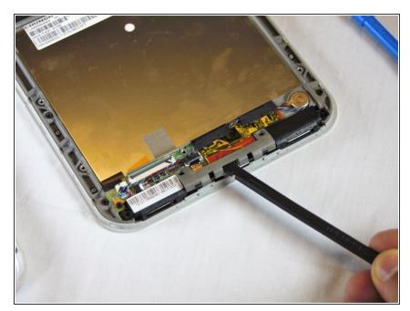
Using the spudger, gently pry up on the reinforcement bar and remove from the frame.
