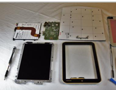
When the frame is separated and loose, Lift from the top and pull the frame off the front glass, setting the glass aside.
