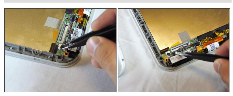
Use the fine pointed tweezers to carefully remove the 2 no-fuss speaker connections.
