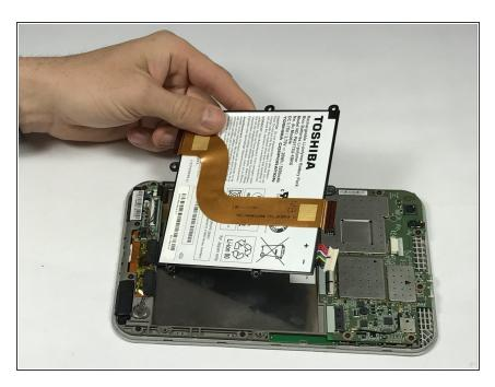
Battery will lift out of the device.
