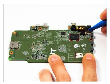
Use small plastic opening tool to pry front facing camera flat top connector from the motherboard
