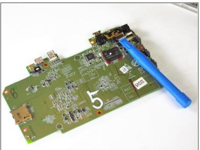
Use small plastic opening tool to pry rear facing camera flat top connector from motherboard.
