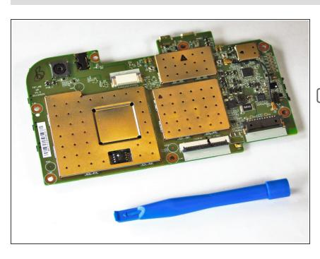
Upon acquiring a new audio jack, use the soldering iron to solder the six connection ports into the motherboard.
