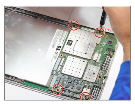
Remove the 4 – 4.5 mm screws from the motherboard assembly.
