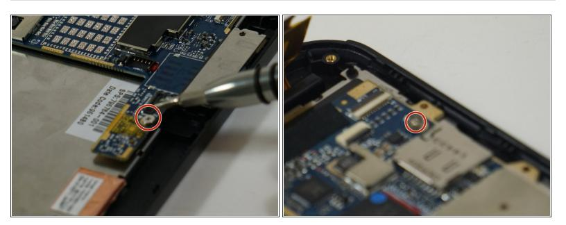
Remove the two 2 mm Phillips 000 screws from the motherboard.
