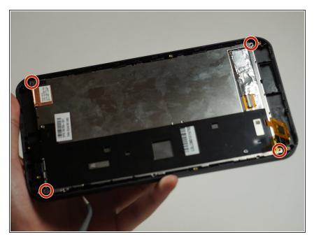
After removing the motherboard, unscrew the four 2.5 mm Phillips 000 screws from the display panel.
