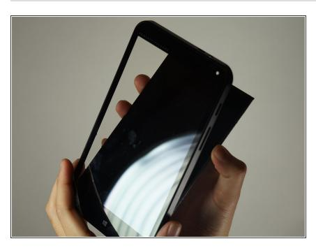
The screen should now just come right off. Be sure to catch any broken bits if the screen is damaged.
