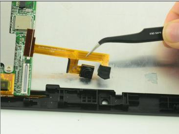
• Use tweezers to lift the camera assembly away from the device.
