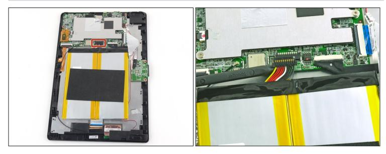
Use a spudger to disconnect the black bundled cable connector from the motherboard.
