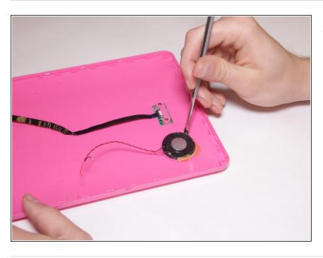
Use a metal spudger to pry out the speakers from its housing.
