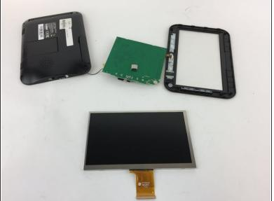
• The LCD monitor will easily come out of the front casing of the monitor.
