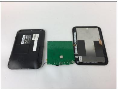
Flip the back panel and motherboard over to reveal the back of the LCD monitor
