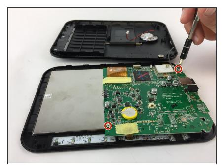
Remove the two 5mm Phillips #1 screws that are holding the motherboard in place.
