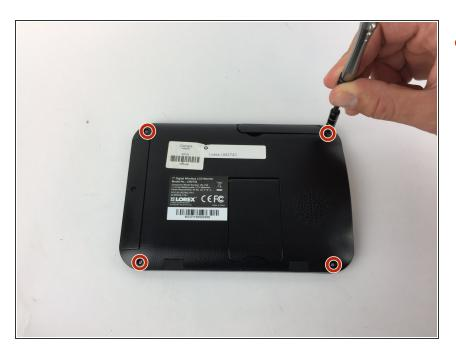
Remove the four 6mm Phillips #1 screws on the back of the LCD monitor.
