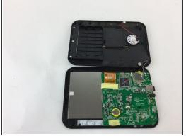
• Locate the motherboard and carefully pull the red and black speaker wires out of their harness.
