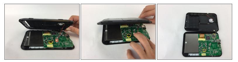
• Locate the motherboard and carefully pull the red and black speaker wires out of their harness.
