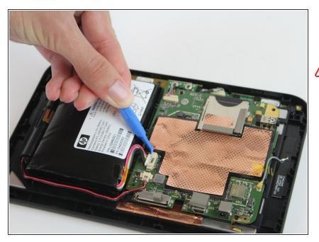
Disconnect the battery clip with a plastic opening tool.
