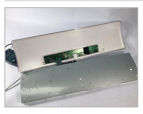
Take the screws off the back of the keyboard to enter the center of the keyboard.
