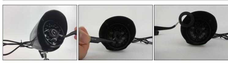
• Remove the foam ring around the lens with <u>tweezers</u>.
