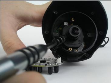
• Use the Phillips #000 to remove the three 3mm screws on the face of the camera lens
