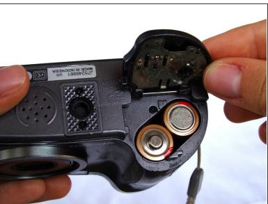
Lift tab up to open battery compartment.
