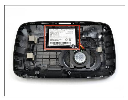
After opening the device and removing the motherboard, you will see the battery attached to the frame.
