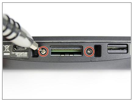
Unscrew the two 3mm screws at the base of the device using the Torx T5 screwdriver.
