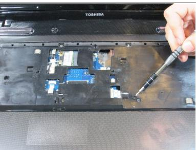
Remove five 5mm screws with the screwdriver.
