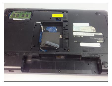
Take out the HDD and leave the connector in the laptop
