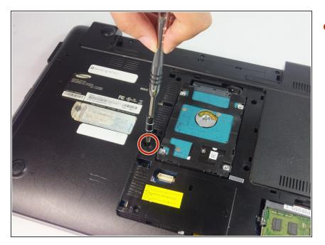
Remove the 4mm Phillips #0 screw using a Phillips #0 screwdriver.
