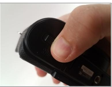
Pull the switch on the bottom of the camera back with your thumb.
