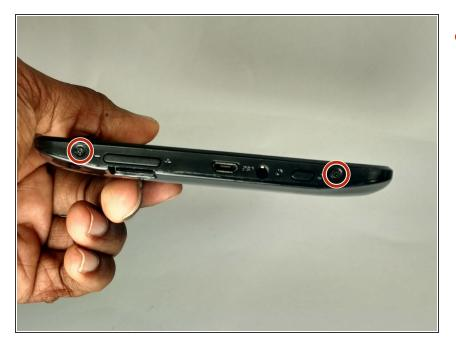
Use a Phillips 00 bit to remove two 3mm screws from the bottom of the tablet.
