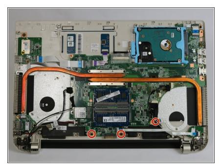
Remove the three 4 mm Phillips #1 screws holding the motherboard in place.
