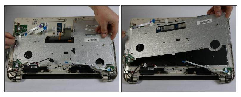
Carefully lift the keyboard retaining plate away from the laptop making sure not to damage any connectors.
