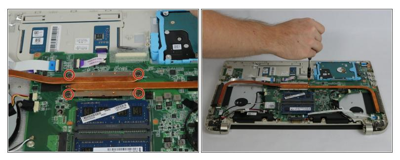
• Remove the four 4 mm Phillips #1 screws mounting the heat sink to the motherboard.
