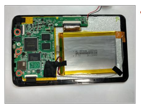
Use a Phillips 00 bit to remove 3 screws from the top of the tablet.
