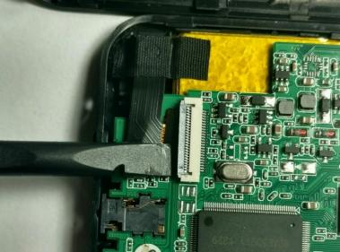
Disconnect three ribbon connectors from the circuit board with the nylon spudger.
