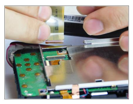
With the small retaining white flap up, remove the LCD screen ribbon cable from the motherboard by sliding it out.
