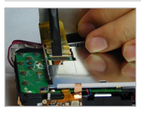
Use the spudger to lift up the small white retaining flap on the motherboard that is connected to the LCD screen's ribbon cable.
