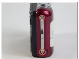
• Remove the six(3.93mm screws) on the outside of the camera using a Phillips 00 screwdriver.
