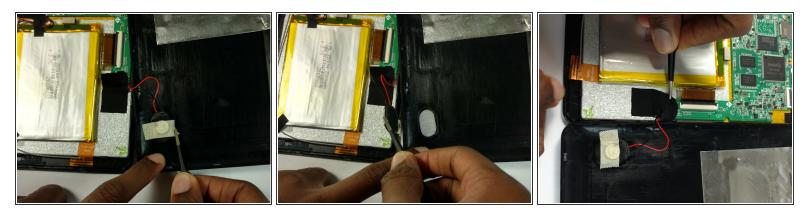
• Using tweezers, carefully remove the tape covering the speaker.
