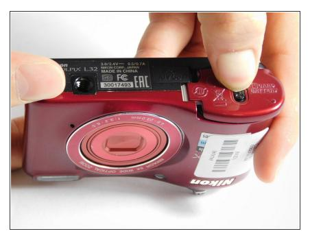
Slide the lock button on the battery compartment away from you while sliding the battery compartment door to the right to open the battery compartment door.
