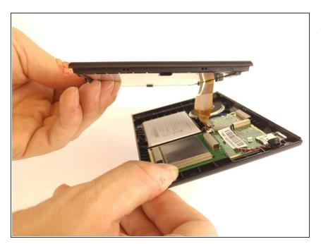
• Once the seam is completely separated, you can lift the back away from the screen easily.
