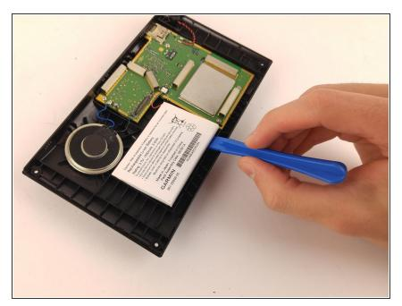
• The white battery is attached to the casing with an adhesive. It should be easy to pry the battery up with a prying tool.
