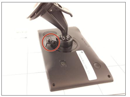
Remove the stand by pushing down on the tab and pulling the round, plastic piece away from the Garmin unit.
