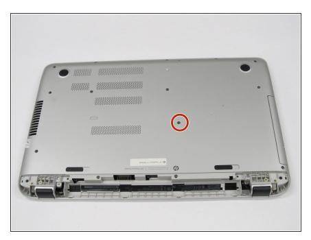
Remove one 7 mm screw with a Phillips #1 screwdriver.
