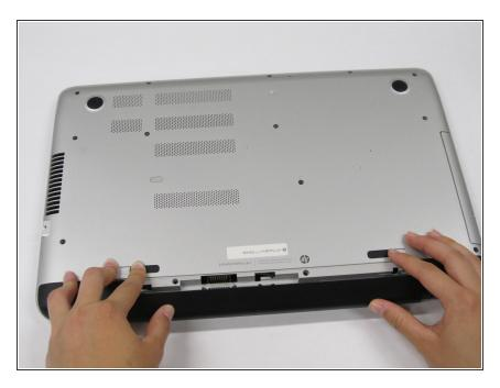
Pull the battery out towards you while your fingers are still holding the latches in place.
