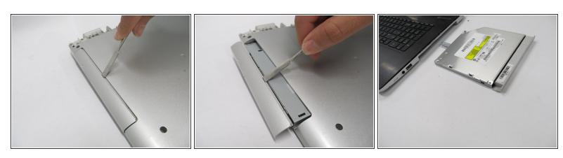
• Use a metal spudger to push the CD drive out of its slot for removal.
