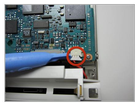
Pull the power cable from the socket located above the upper right side of the battery harness.
