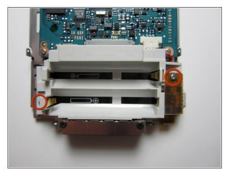
Using a Phillips #0 screwdriver, unscrew the two screws towards the bottom sides of the Sony Clie to remove the battery harness.
