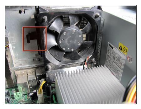
Locate the release clip on the side of the fan and hold it down with your thumb.
