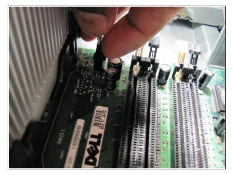
Follow the power cable to the motherboard connection and remove it by pressing down on the clip.
