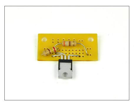
Insert the leads of the 240 Ω resistor through the holes indicated in step
