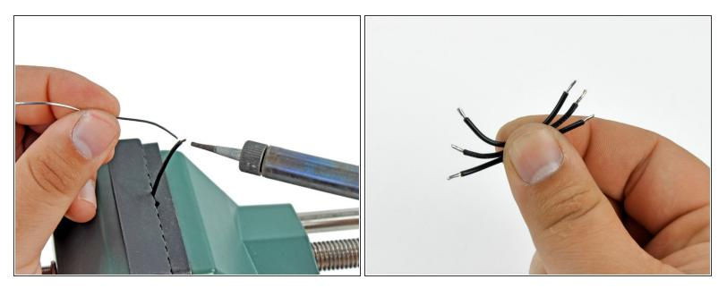
• Secure a wire and pre-tin both of its ends. Repeat for the remaining two wires.
