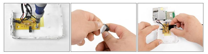
• Secure the PCB to the upper case half using the original 5.38 mm #1 Phillips screw and the included washer.
