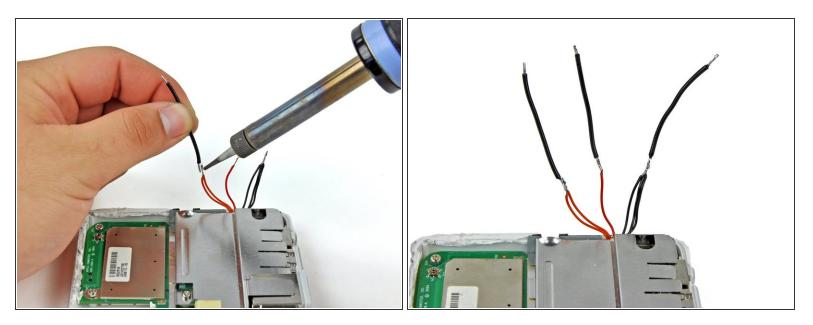
Align the pre-tinned section of the cut wire with one of the lower case power wires. Melt the two
