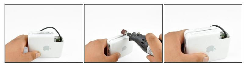
• There are likely large burrs (shredded plastic bits) on the edges of your case from cutting it open. For ease of joining the case halves, it is recommended that you smooth the edges by de-burring them. A dremel tool with a sanding bit, a sanding block, or a knife will work for this process.
