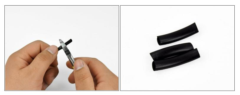
• Cut the included heat shrink tubing into 3 equal length pieces.
