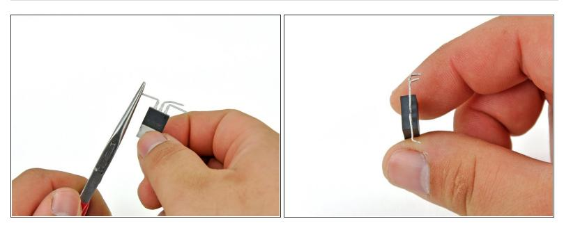
• Use needle nose pliers to bend just the tips (approximately 2 mm) of the pins 90° up so that they are pointing the same direction as the IC face.
