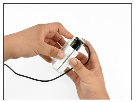
Put the case halves together. Be careful not to pinch the 3 power leads, and be sure to route the power supply cable out of the opening in such a way that it won't put tension on any of the PCB components.
