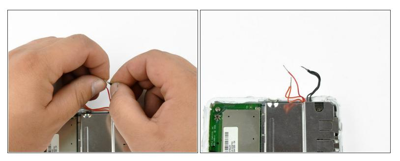
• Twist the exposed ends of the same-colored wires together.
