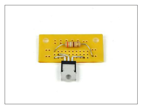
Insert the leads of the 390 Ω resistor through the holes indicated in step 7. This resistor will have an orange, grey, brown and gold band on it. The direction of the resistor does not matter.
