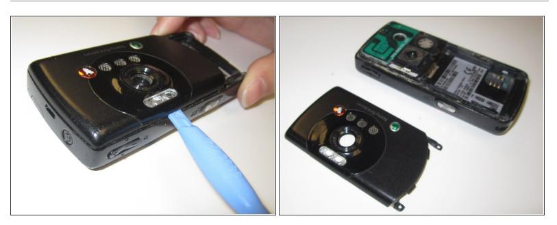
Remove the Back (camera side) Faceplate with the blue hand-wedge
