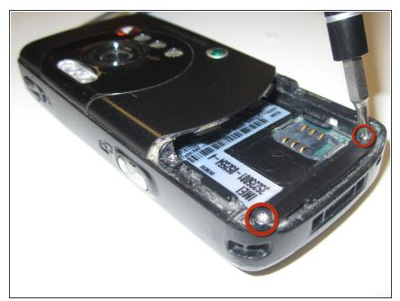
Remove the two outer screws using a T-7 head for a screwdriver
