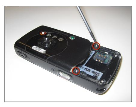
Remove the two smaller inner screws with the Mini-Phillips screwdriver head
