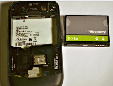
Pinch the battery at the grey semi-circles on the top left and top right corners of the battery using your fingers and remove it from the device.
