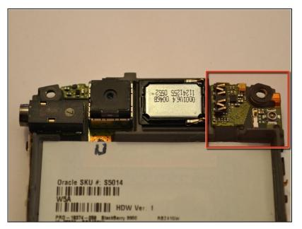
Replace the entire center piece of the case to replace the antenna.
