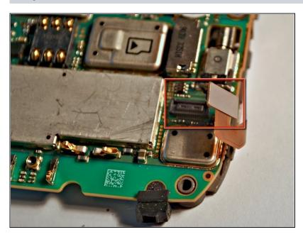
Carefully disconnect the ribbon cable located on the bottom right of the motherboard.
