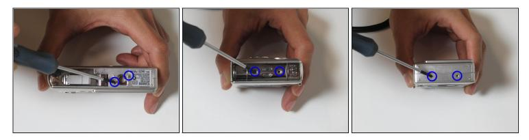
• Using the screwdriver, carefully remove the exterior screws and set them aside to avoid misplacing them.
