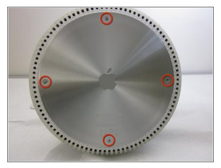
Loosen the four Phillips #0 screws.
