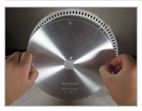
Carefully remove the base access panel.
