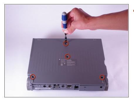
Use a T10 torx screwdriver to remove the four, 18mm long screws from the lower case.
