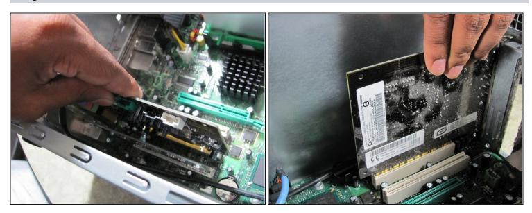
• Grasp the Sound Card and pull it up and out of it's slot.
