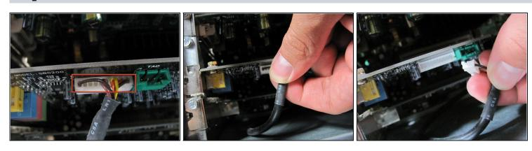
• Locate and remove the white connector on the sound card by pulling on the black cable.
