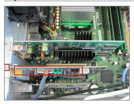
Locate the Sound Card and the screw attached to the Sound Card as shown in the picture.
