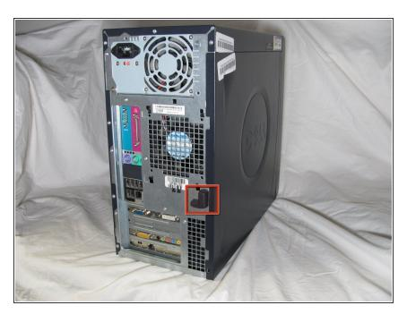
Locate the case cover latch on the back of the computer.
