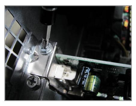
Remove the 8.9 mm screw by using a Phillips #2 screw-driver.
