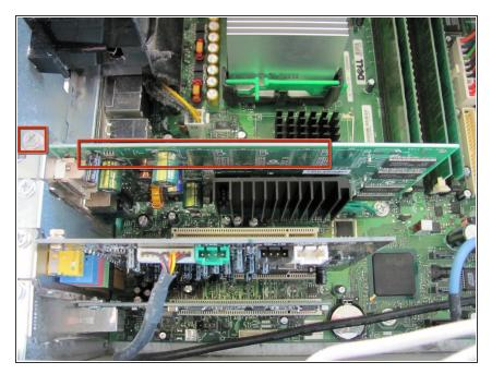
Locate the Video Card and the screw attached to the Video Card as shown in the picture.
