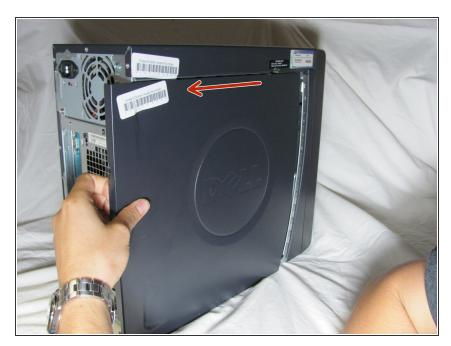
Grab the edge of the panel and slide it away from the case until it is removed.
