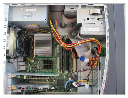
(i) Lay the computer flat so that you are looking down on all of the components.
