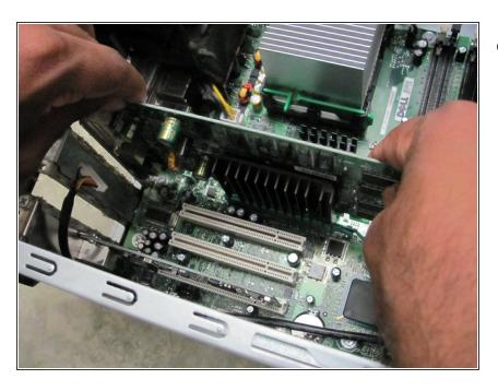
Pull the remainder of the card up and out of it's slot.
