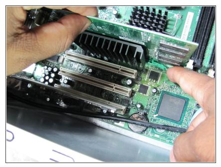
Push down on the green clip located by the bottom right corner of the video card while simultaneously pulling the card up with your other hand.
