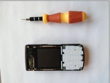
Use the T6 Torx screwdriver to remove the six 15 mm Torx screws.
