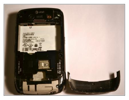
Using a small plastic opening tool, remove the lower rear cover.
