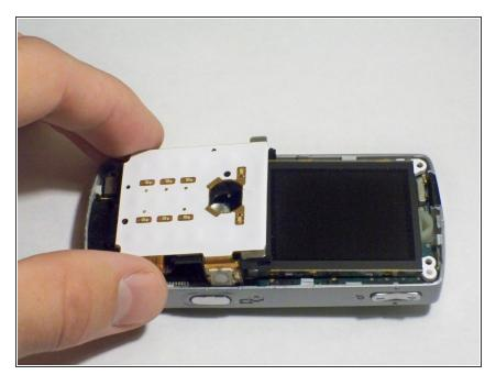
Gently lift the base of the keypad to remove it.
