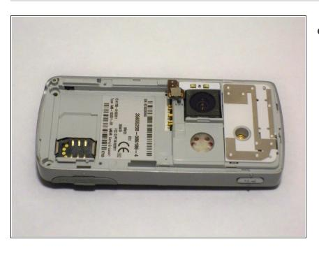
Remove the casing to expose the camera's components.
