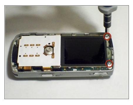
Remove the screws holding the screen in place.
