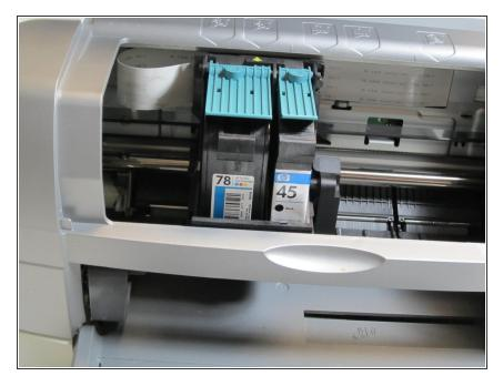
The ink cartridge should be located in the center of the printer. The cartridge on the left holds the color ink and the cartridge on the right holds the black ink.
