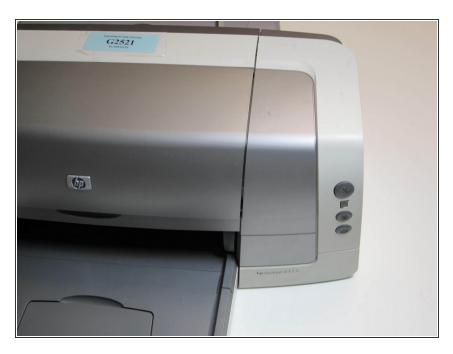
• Check to see if the printer is on. You can do this by identifying whether or not the bottom button on the right face of the computer is green. If button is green, proceed. If the button is not green, turn the printer on, and then confirm the bottom button is green.
