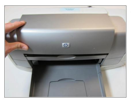
Finish installing new cartridges by shutting the front panel. The printer should react by moving the cartridges back to the their original resting position.
