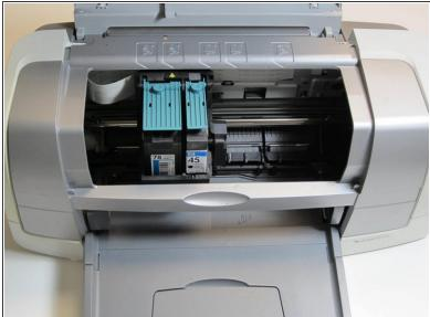
• Lift the front panel to gain access to the inside of the computer. Upon opening the front panel, the printer should respond by moving the print cartridge towards the center of the printer.
