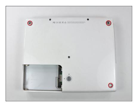
Remove the three newly-revealed Phillips screws.
