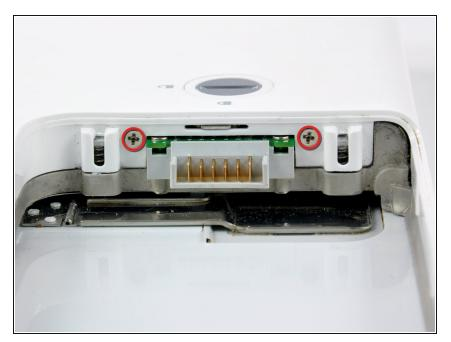
Remove the two 4.5 mm Phillips screws on either sides of the battery contacts.
