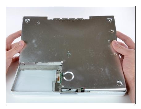
• Lift the bottom shield off.
