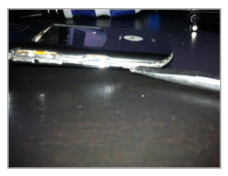
After removing the screws, use a flat surfaced tool to take the face-screen off.
