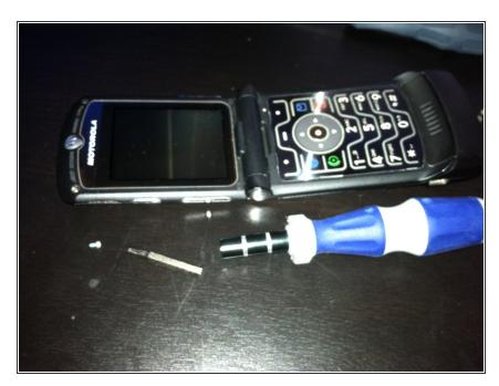
Unscrew the four screws located around the face plate using a 1.5mm Hex tool.
