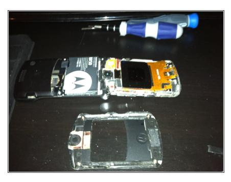
After securing the face-screen into the casing, place the face screen cover back on.
