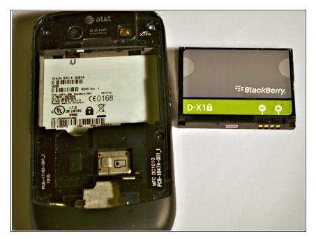
Open the rear panel to expose the battery and the chassis assembly.
