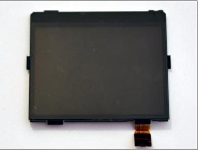
• Carefully pry at the sides of the screen until the display assembly is free. Remove the display from the motherboard unit.
