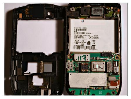
Remove the midframe from the back of the phone, which should now be free after removing the screws. The green motherboard should now be exposed.
