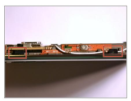
Remove the front-cover by carefully prying the side release tabs, located on the side of the phone.
