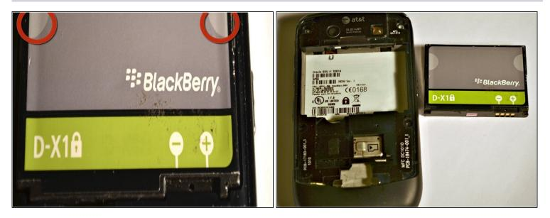
• Pinch the battery at the grey semi-circles on the top left and top right corners of the battery using your fingers and remove it from the device.
