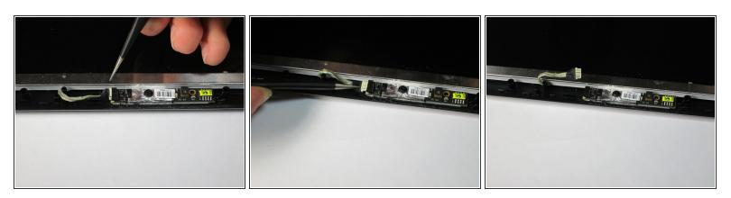
• Disconnect the webcam data wire using tweezers.
