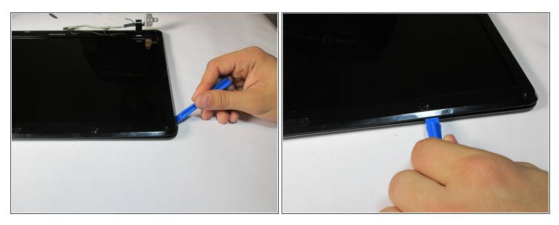
• Use the plastic opening tool to pry the screen housing.
