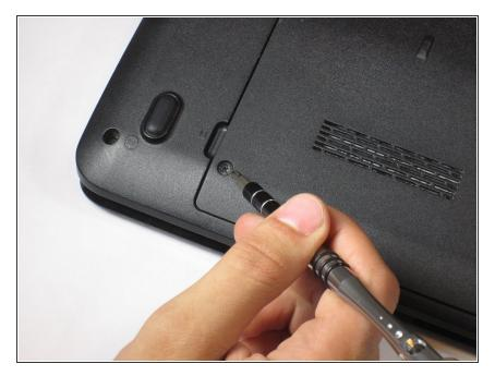
Remove the single captive screw on the back panel with your Phillips #1 screwdriver.
