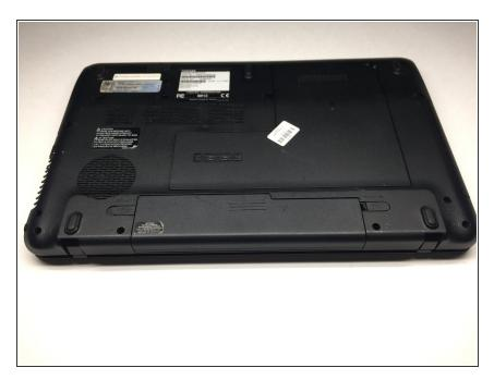
• Flip the laptop upside down. Locate the two latches on both sides of the battery.
