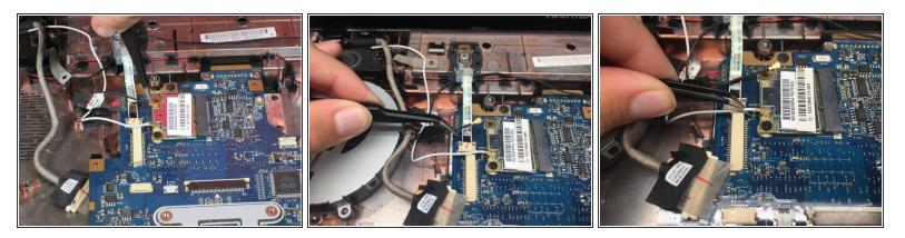
• Lift the black connector with tweezers and repeat the same action for the white connector.
