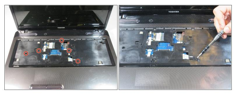
• Remove five 5mm screws with the screwdriver.
