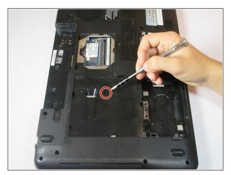
Remove the single 5mm Phillips #1 screw using the screwdriver.
