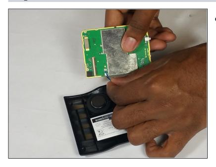
Use a soldering tool to desolder the connection to the motherboard. Refer to the iFixit Soldering guide to see how
