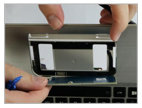
Once the adhesive is separated enough from the touchpad, peel it back and remove it.
