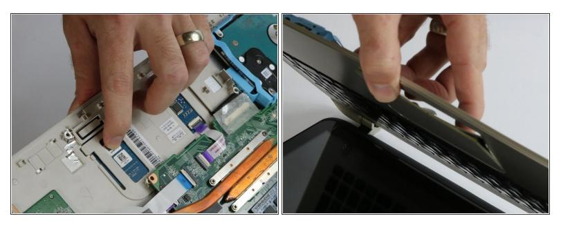
• Gently push the back side of the touchpad in order to create a gap on the top side of the touchpad.
